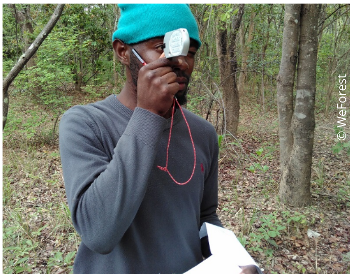
WeForest's extensionist Donnell measures the tree height with a clinometer.
