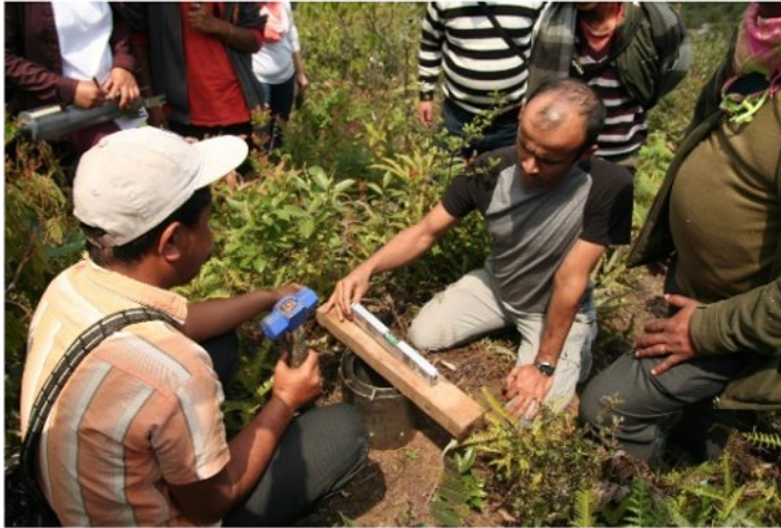
Figure 5. Learning to use the double ring infiltrometer (left) and practicing rainfall data recording (right).
