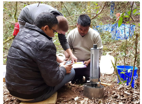
Measuring rainwater infiltration.
