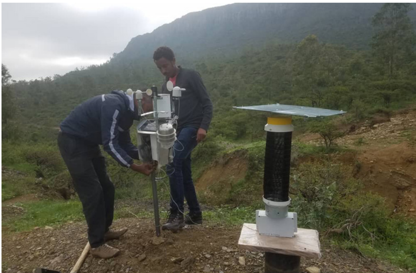
Figure 2: Building the automated weather station provided by Kings College London & Ambiotek.
